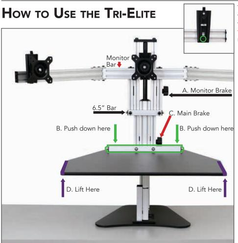
To move the mount horizontally closer or farther apart, simply loosen the bolt attached to the horizontal monitor rail (B) by a single turn with a 5/32 allen wrench. Once you have reached the desired position tighten the bolt.
