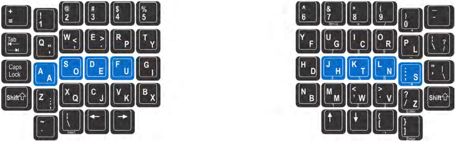
Fig 12. QWERTY-Dvorak dual-legged keycaps for Advantage2
