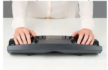
Fig 7. Closer placement of function keys & integrated palm support
