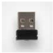
This small, wireless receiver can be securely stored in the magnetized battery housing when not in use. (Wireless only).
