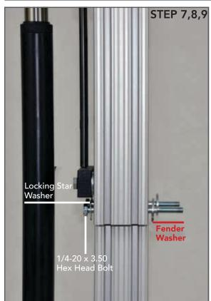
**Step 7:** Put (1) Locking Star Washer{I} on each of the  $1/4 - 20 \times 3.50$  Hex Head Bolts{B}.
