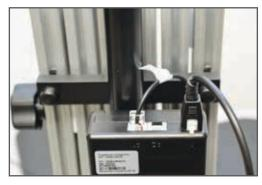
**Step 6:** Connecting the controller from the work surface and cable to the actuator. Connect the cable from the work surface that holds the controller into port "A1". Connect the cable from the actuator into the right port labeled "1" as shown above.
