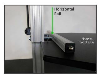
Step 8: Lift the Work Surface up and align the holes in the Horizontal Rail with the (2)  $1/4-20 \times 3.50$  Hex Head Bolts. Push the Work Surface onto the Hex Head Bolts until the threads of the bolts come through the Horizontal Rail.
