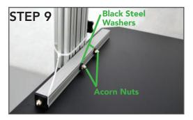
**Step 9:** Put (1) Black Washer{G} and (1) Acorn Nut{E} on the end of each of the Hex Head Bolts. Using the 7/16 wrench{H} tighten the Acorn Nuts securely. After you have the work surface secure, you can cut the zip tie holding the assembly together.
