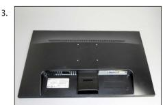
Remove the Base From Your Monitor and Lay it Face Down on a Soft surface
