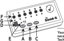
The function of a switch paired with a stand-alone receiver is implicit and does not need to be programmed. All six channels of SEND-6 will operate the receiver, irrespective of their function settings. This allows a number of co-operative exercises to be devised.
